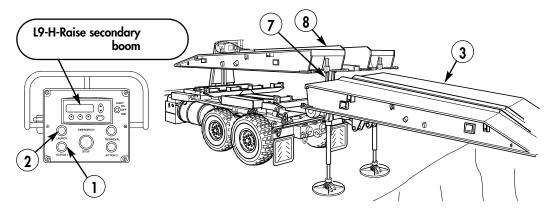
33. Depress LAUNCH button (2) to confirm and step into next function.
