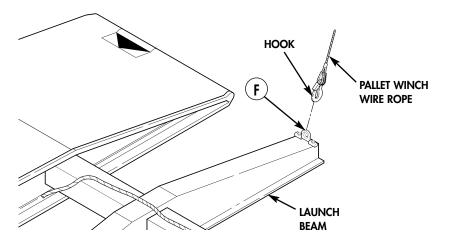
**ANCHORING EYES** — There is an anchoring eye on the outboard side of each bridge quarter at the ramp end. Once the bridge is emplaced over a gap, anchoring straps are connected to the four corners of the bridge at each anchoring eye. The four anchoring eyes are used for bridge anchorage only.
