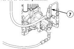
BYPASS VALVE, OPEN POSITION
