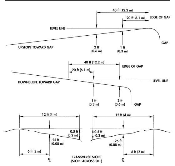
Figure 4. Shore Slope Measurement.
