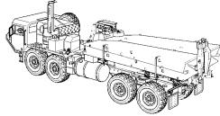
Figure 1. Rapidly Emplaced Bridge on CBT, Typical.
