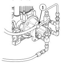
**BYPASS VALVE, CLOSED POSITION**
