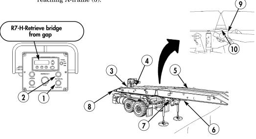
28. Depress RETRIEVAL button (2) to confirm and step into next function.
