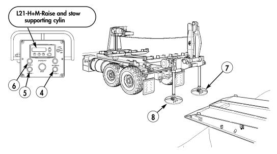
57. Depress and hold ACTION 2 button (4) and ACTION button (5) simultaneously to L21-H+M-RAISE AND STOW SUPPORTING CYLINDER, and observe right supporting cylinder (7) and left supporting cylinder (8) retract. Release buttons (5) and (4) when fully retracted.
