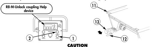
Ensure all coupling help device levers and both upper coupling lock levers are disengaged from lock receptacles before proceeding to next function; use soft-nosed hammer only. Failure to comply may result in damage to equipment.
