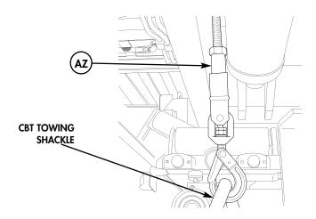
PALLET HOLD-DOWN BAR, CONNECTED TO CBT
