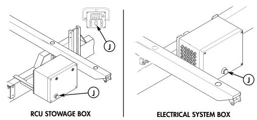
**RCU STOWAGE BOX LOCKS** — There are two locks on the front door of RCU stowage box. To open door, position RCU stowage box key on square and turn key to the left on each lock. To lock door, close door tight against stowage box and turn key to the right on each lock. Key is stowed in adjacent pallet toolbox.
