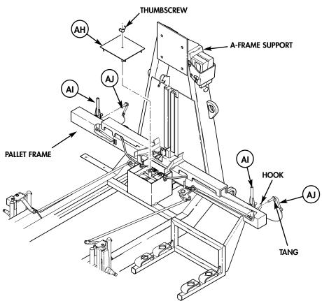
SUPPORTING WHEELS HYDRAULIC PUMP HANDLE — This removable handle is used as an extension lever to manually operate the hydraulic pump. The pump handle is stowed on A-frame. To remove, release strap and lift handle off mounting stud. To operate pump, slide handle on pump lever and move handle back and forth.
