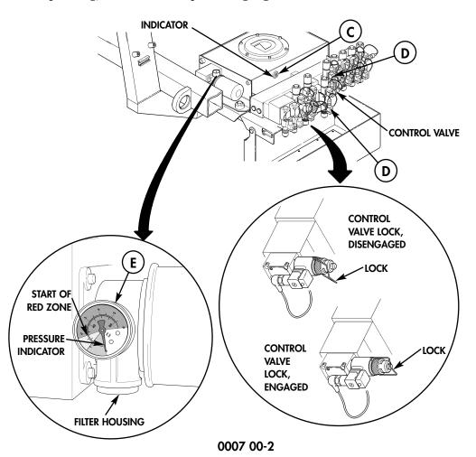
**PALLET HYDRAULIC PUMP BYPASS VALVE LEVER** — Prior to starting LPU, determine weight of oil in pallet hydraulic system and its ambient temperature range. Refer to WP 0025 00. To operate, turn lever to open bypass valve; lever should point down. Once LPU engine is running, close bypass valve; lever should point to left. The bypass valve should remain open when operating pallet hydraulic system off CBT hydraulic pump.
