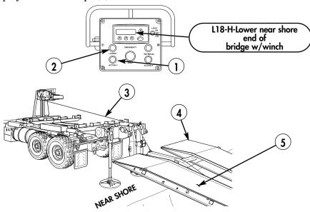
51. Depress LAUNCH button (2) to confirm and step into next function.
