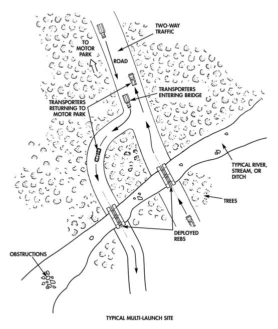
Figure 2. Bridge Assembly Site Layout for Multi-Launch Site.
