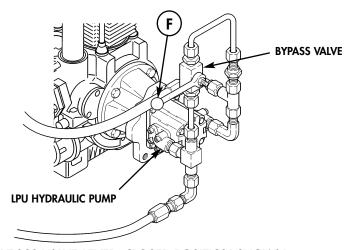
BYPASS VALVE LEVER, CLOSED POSITION SHOWN
