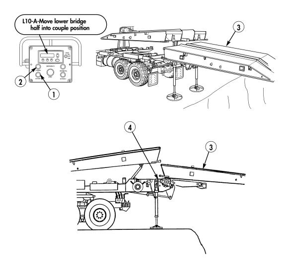
35. Depress LAUNCH button (2) to confirm and step into next function.
