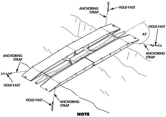
Perform steps 9 through 15 to remove anchorage from bridge.
