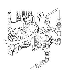
**BYPASS VALVE, CLOSED POSITION**
