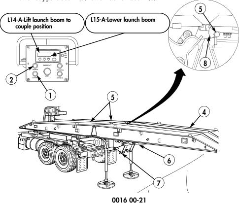
45. Depress LAUNCH button (2) to confirm and step into next function.
