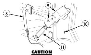
High idle switch must be in the OFF position prior to engaging PTO. Failure to comply may result in damage to the vehicle transmission.
