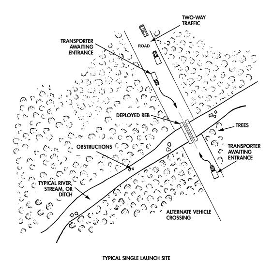
Figure 1. Bridge Assembly Site Layout for Single Launch Site.
