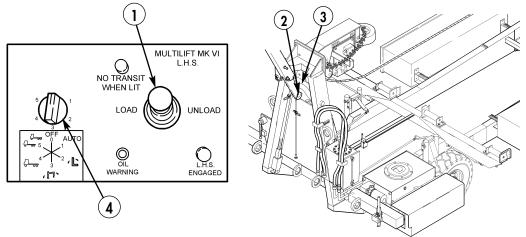
15. Turn LHS MODE SELECT switch (4) to No. 1 (AUTO) position or REMOTE CONTROL (late model CBTs).
