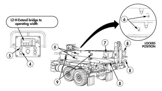
14. Depress LAUNCH button (5) to confirm and step into next function.
