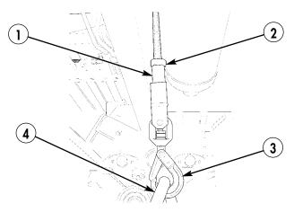
11. Place both hold-down bars (1) in stowed position on pallet cleats (5).
