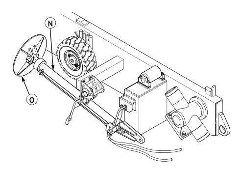
SUPPORTING CYLINDER, RAISED AND SECURED
