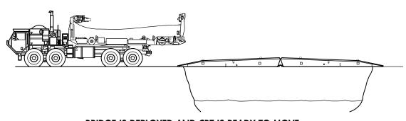
BRIDGE IS DEPLOYED AND CBT IS READY TO MOVE.
