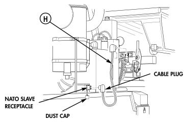
MAIN POWER SWITCH — The main power switch connects/disconnects electrical power to pallet electric system from pallet batteries and CBT batteries, whichever are in use. To operate switch, remove dust cap and insert key in switch. Turn key to the right to turn on power. Turn key to the left to shut off power.
