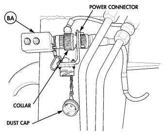
WINCH EMERGENCY SWITCH, CONNECTED
